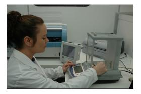
Equipment & Instrumentation: Denver Inst. A-250 & PI-114 Analytical Balances, SIMCO 500 Static Control Air Gun, U-Shaped Static Electrode
